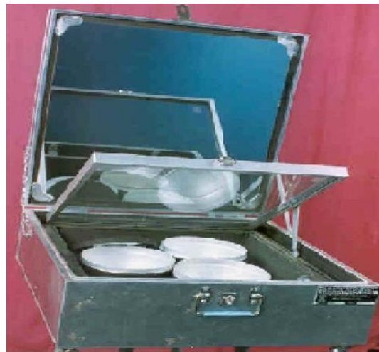
Figure 2: An overview of a box-style cooker created by Nahar [3] that uses hot oil as a thermal storage medium
