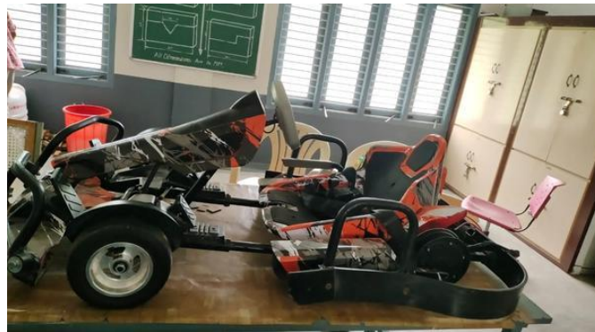
FIG 4:- SIDE VIEW OF FABRICATED ELECTRIC VEHICLE
