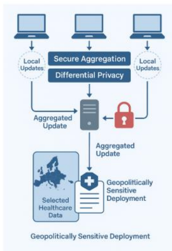
Figure 2: Secure federated learning architecture using cryptographic protections. Clients encrypt model updates using homomorphic encryption and secure aggregation protocols before sending them to the aggregator. Even if the aggregator is compromised, individual updates remain protected. This decentralized design supports deployment in geopolitically sensitive regions such as EU Cyber Shield or cross-border healthcare networks, where sovereignty constraints prevent centralized control. Gradient clipping and noise scaling mechanisms further enhance data privacy by mitigating the risk of sensitive input reconstruction.
