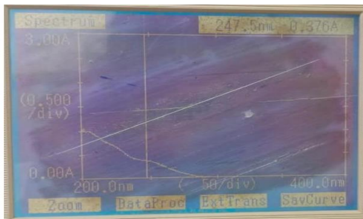
Figure 1: UV absorption spectrum of losartan potassium in distilled water showing the maximum absorption at 247 nm.
